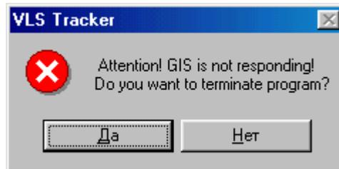
Fig. 37 Request for closing GIS if hang condition is detected
