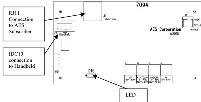
**Installing the 7094 in the Subscriber Unit (AES 7058):**
