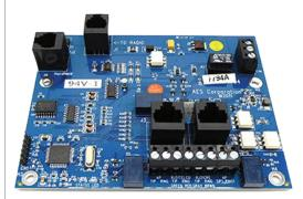
The 7794A AES-IntelliPro Fire is an add-on module for IntelliNet 2.0 subscribers that enables transmission of full alarm zone data from an alarm panel to a central station over an established AES mesh radio network.
