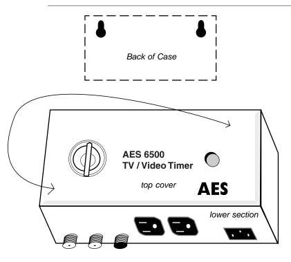
For Wall Mounting - Screw holes are provided on the rear of the case to mount this device on a vertical surface (do NOT use rubber feet).
