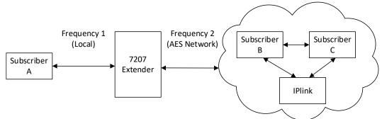
The optimum location for the extender will provide good connectivity to the existing AES RF network, and will be in relatively close proximity to the subscriber location, for example, within the same building. A typical installation might have an extender installed near the roof of a building to provide connectivity with a subscriber located in the basement.
