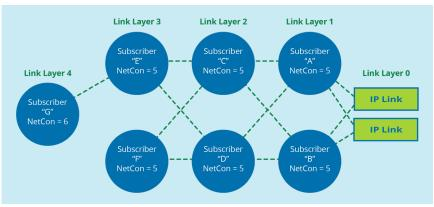
In the graphic above, you can see that the IP Link is a Link Layer of 0. This will always be the Link Layer value for an IP Link. Subscriber Unit A has a Link Layer of 1 as it is 1 'hop' from the IP Link. Subscriber Unit C is a Link Layer of 2 because it is 2 'hops' away from an IP Link. This logic continues down the chain.
