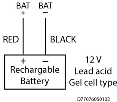
**Figure 3. Connecting the Battery Backup**
