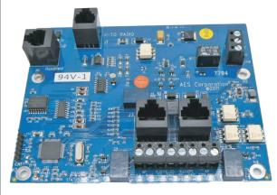
The 7794 AES-IntelliPro Fire<sup>™</sup> is an add-on module for AES Subscribers that enables transmission of full alarm zone data from an alarm panel to a central station over an established AES-IntelliNet network.
